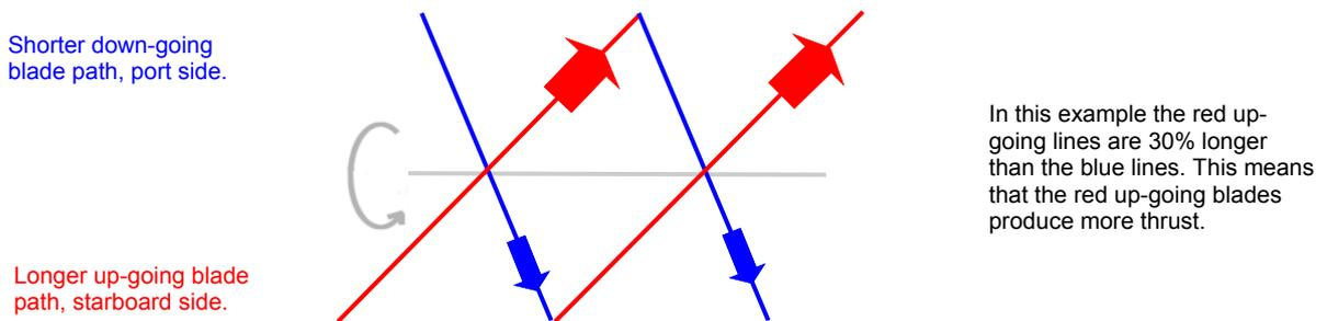
The thrust from the starboard side is stronger than the thrust from the port side, therefore prop walk yaws the stern to port.
