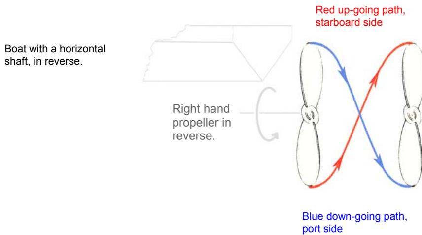
The schematic below shows the cylindrical paths of the blades as a flat representation during one rotation.
