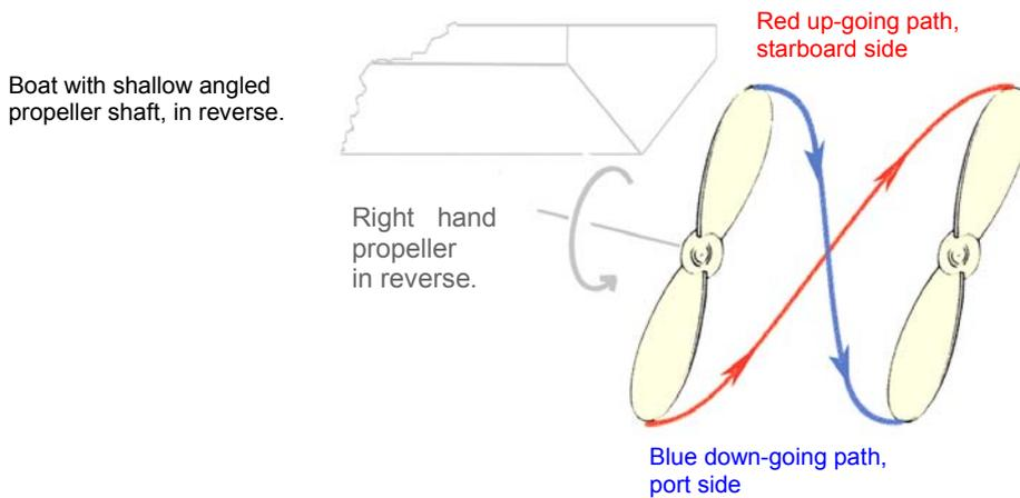
The schematic below shows the cylindrical paths of the blades as a flat representation during one rotation.
