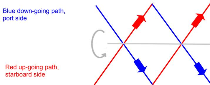
The thrust from the port and starboard sides is equal and in line with the propeller shaft; there is no prop walk.
