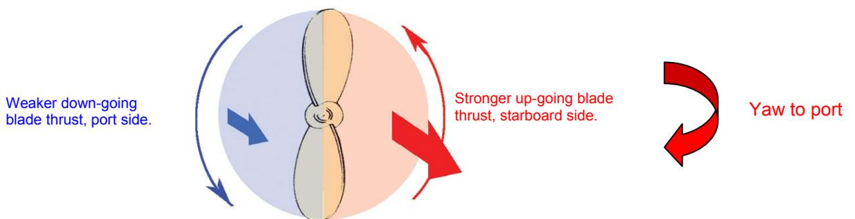
Prop walk is caused by the angle of the propeller shaft to the water surface; if there is no angle, then there is no prop walk. For an increase in either the diameter or pitch of the propeller the effect is increased.
